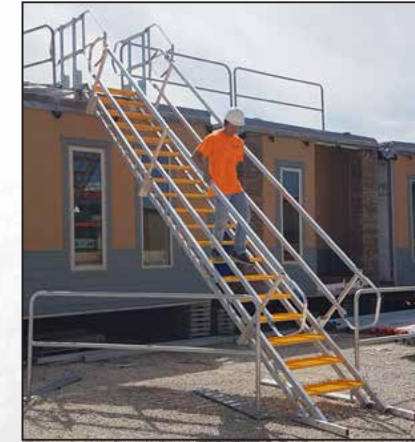
PT# 15102; Para-Stair Assembly, 16-NS Consists of 15136 (1X), 15135 (6X), 15137 (1X), 15085 (4X), 15141 (1X). Maximum (60°): Height 176.50" (4483mm) x Offset 122.63" (3115mm). Minimum(30°): Height 102.00" (2591mm) x Offset 196.50" (4994mm).
