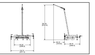
PRO-7 Sky-X-Stand systems are a counter weighted (stell bins must be filled with concrete) hitch mounted (units must be attached to vehicles during use) anchor point.
